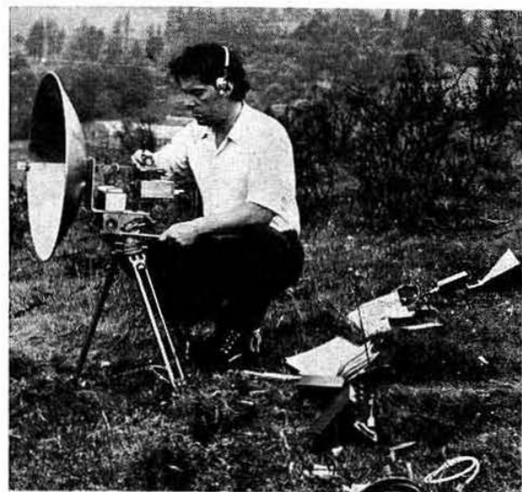
That well-known microwave enthusiast GM3OXX seen operating his 3cm portable gear in the county of Kinross. This is the equipment which achieved the British 3cm record distance of 243km earlier in the year. The object fitted with a horn seen in the right background is an even smaller portable 3cm transceiver
