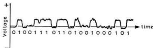
Fig 2. The pulse train of Fig 1 with attenuation, noise and distortion after transmission over an imperfect signal path
